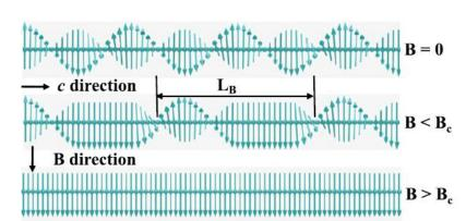
Magnetic structures coupled to transport: aligning spins lowers resistance
