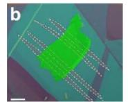
Thin Crl<sub>3</sub> as tunnel barrier between graphene contacts
