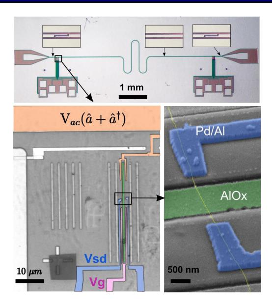
Stamped single wall carbon nanotube quantum dot coupled to microwave photons
