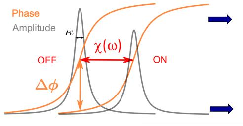
The charge susceptibility of a QD connected to its leads shifts the transmission
