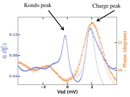
Kondo resonance is 'transparent' to photons while charge peaks visible.
