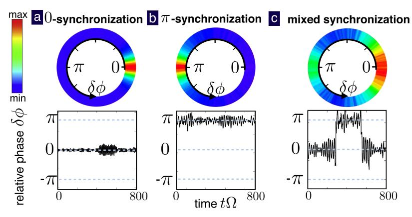
phase distribution and typical quantum trajectories for two coupled (optomechanical) limit-cycle oscillators
